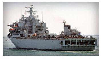
when unloaded would be excessive making her motion at sea uncomfortable or even dangerous. Therefore, her superstructure is deliberately heavily built (weighing some 800 tons), and she has 1,800 tons of concrete ballast carried in former hatch covers.
